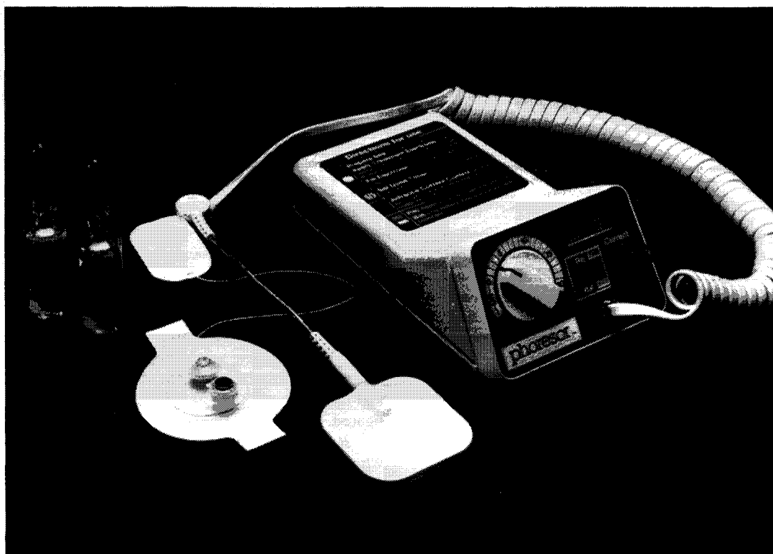
Fig. 7. The control unit and the electrode system of the Iontophoretic device. (Phoresor) manufactured by Motion Control, Inc., Salt Lake City, Utah.
